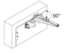
Attach the armset to the mechanism ensuring the pre-loading requirement has been completed.
